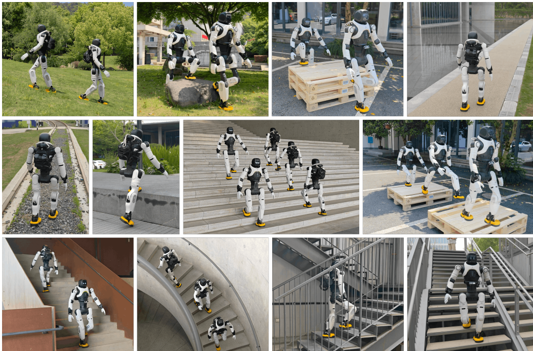
Figure 1: SSR scales surefooted and symmetric humanoid traversal to diverse open-world human environments. Driven by egocentric vision, the robot reliably traverses grassy slopes, stairs of varying sizes and structures, steps onto high platforms, and crosses wide gaps. Throughout long-horizon traversal, it maintains safe foot placement together with coordinated and natural whole-body motion.
