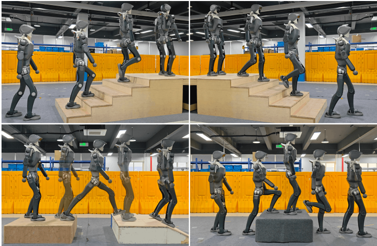
Figure 11: Key frames of cross-platform laboratory deployment on the full-size DEEP Robotics DR02 humanoid. The SSR policy successfully traverses stairs, an 80 cm gap, and a 45 cm platform, demonstrating its cross-platform generalization.
